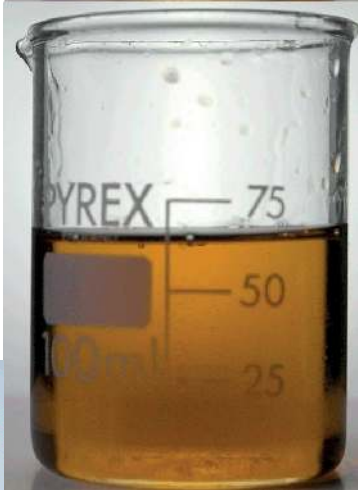
DIESEL BUG SOLUBILIZED INTO THE FUEL
