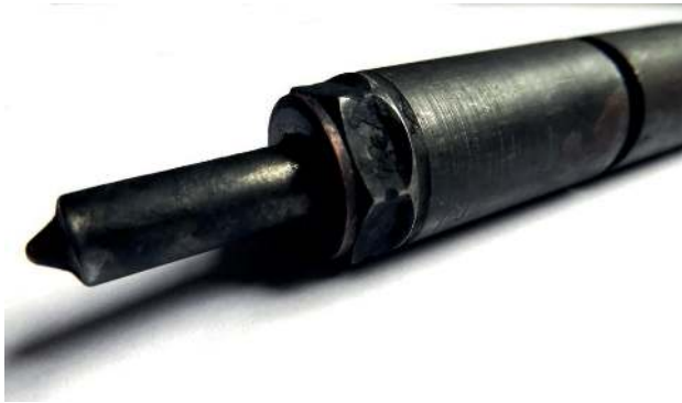
Injector before use of HC24
